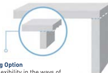
Tile Assembly Visible junction
