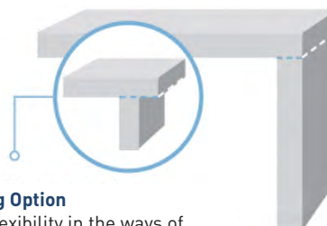
Tile Assembly Visible junction
